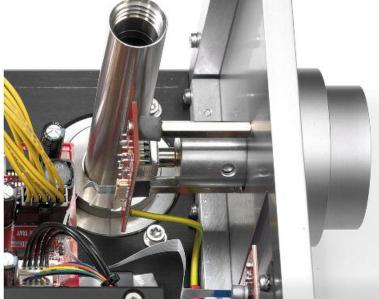
Above: At CH Precision, it is not enough to simply decouple the drive itself from the rest of the device in an ultra complex manner – the toroidal transformers in the power supply unit are also mounted on vibration dampers
